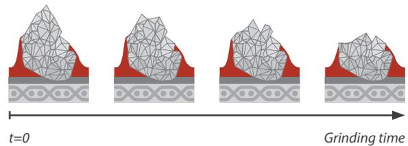
Due to their optimised and thus finer microcrystalline structure, **VSM CERAMICS Plus** series feature an improved self-sharpening effect, which produces much more sharper edges.
